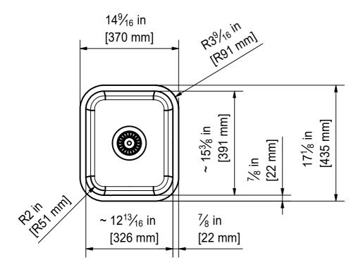
The dimensions of the sink may vary due to the fireclay manufacturing process. Therefore don't use these dimensions as templates for the cut-out. Look at the instructions in the Installation Manual instead.
