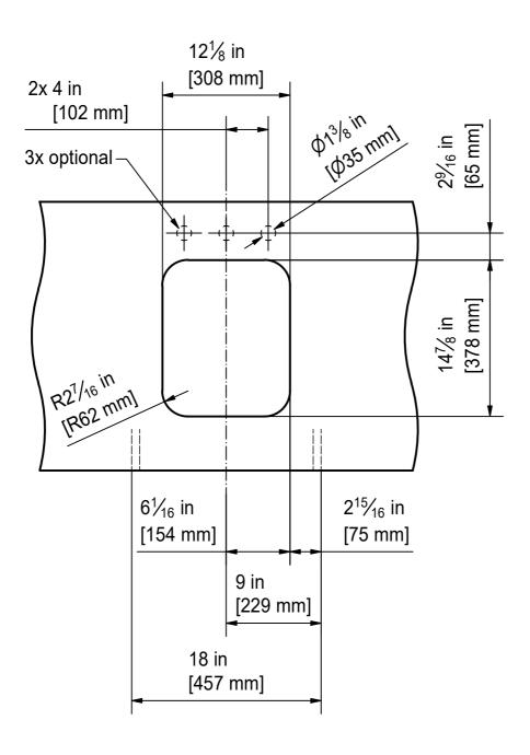
The dimensions of the sink may vary due to the fireclay manufacturing process. Therefore don't use these dimensions as templates for the cut-out. Look at the instructions in the Installation Manual instead.
