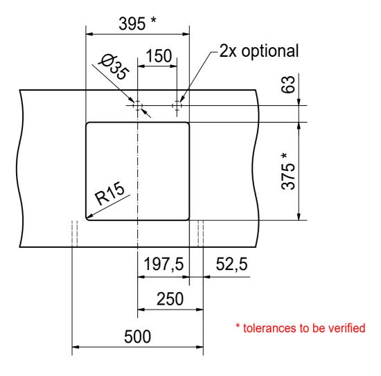
Due to material tolerances, it is recommended to make the cutout based on the supplied sink.
