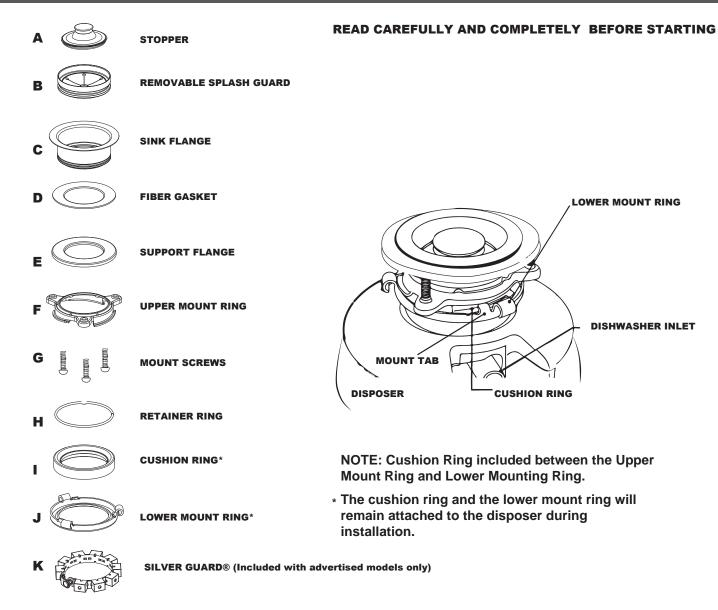
NOTE: The mounting components are assembled out of the box in the same order they will be assembled on the sink, so please pay close attention to the order of the mounting system components before you disassemble them.
