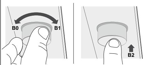
When the dial is turned clockwise the speed increases, passing from:
