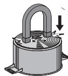
**Note:** Use only cookware with a perfectly flat bottom and suitable for induction cooking zones. Using cookware with an irregular bottom could jeopardise the efficiency of the heating system and prevent cookware from being detected on the cooking zone.
