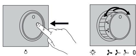
**Lights** - To turn the lights on, press the dial and release it so that it pops out of its housing. To turn the lights off, push the dial back inwards, returning it to the off position.
